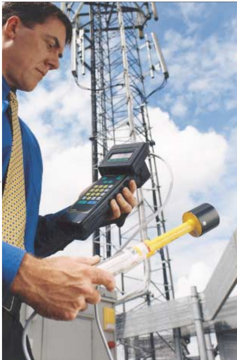
Field tech puts a Narda radio-frequency radiation meter and probe through their paces.
